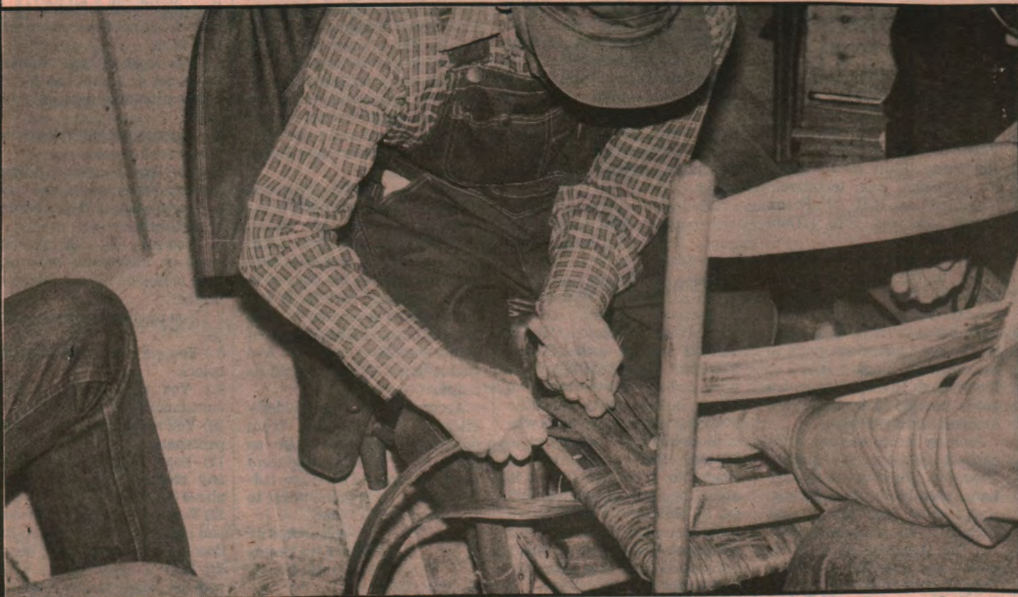
Thornton weaves the second layer of bark on the chair bottom, from left to right, between the strips of bark running from front to back. He uses a knife to push the bark closer together to make the seat sturdier.
